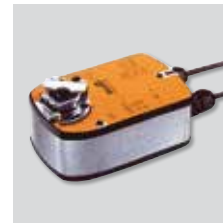
LF 230 S [AC 230V, 50/60Hz] LF 24 S [AC 24V 50/60Hz/ DC 24V] Servo motor with spring motor. 4 Nm. Control signal On/Off.
